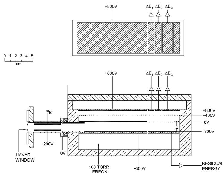
**Figure 7.** The  $^{10}\text{Be}$  detector used at the Australian National University. It incorporates the stopping of  $^{10}\text{B}$  and the measurement of the residual energy of  $^{10}\text{Be}$  within the same gas volume.
