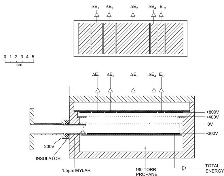
**Figure 4.** A cross section through the multi-element ionization chamber used at the Australian National University for  $^{36}\text{Cl}$ ,  $^{14}\text{C}$  and  $^{26}\text{Al}$  detection. The upper panel shows a plan view of the anode electrode.
