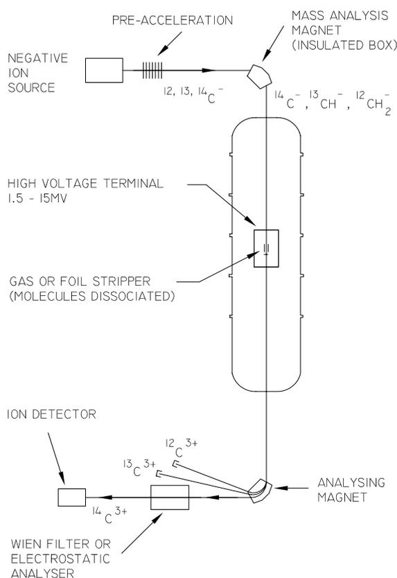
**Figure 1.** The essential features of an AMS system. The first magnet is shown as transmitting mass-14 negative ions. It is also set periodically to transmit mass-12 and mass-13 ions, in which cases the accelerated ions are detected in the off-axis cups after the analysing magnet.
