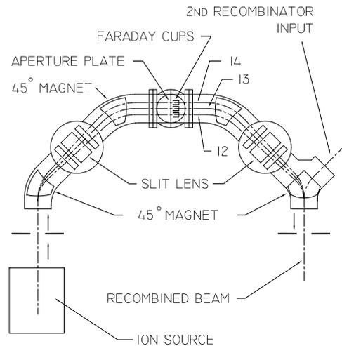
**Figure 3.** The recombinator injection system used by the AMS systems based on the Mk II Tandetrans.
